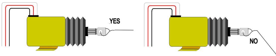
The solenoid cable may be manually pulled while hanging. This will easily release the door latch, which may be manually reset to study the release action caused by pulling the solenoid cable. Keep in mind that a binding solenoid plunger from a sideways pull will not perform properly.
